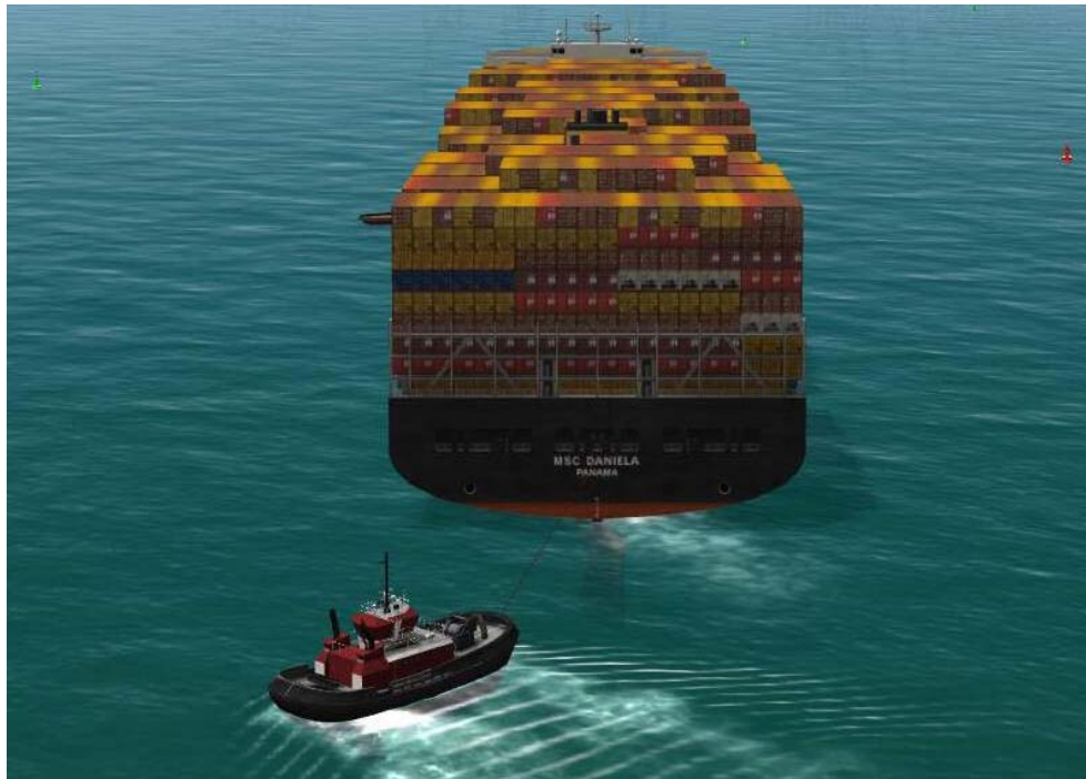
Figure 14: Tug Stalling trying to Accomplish a 90° Direct Pull at Bergen Point
