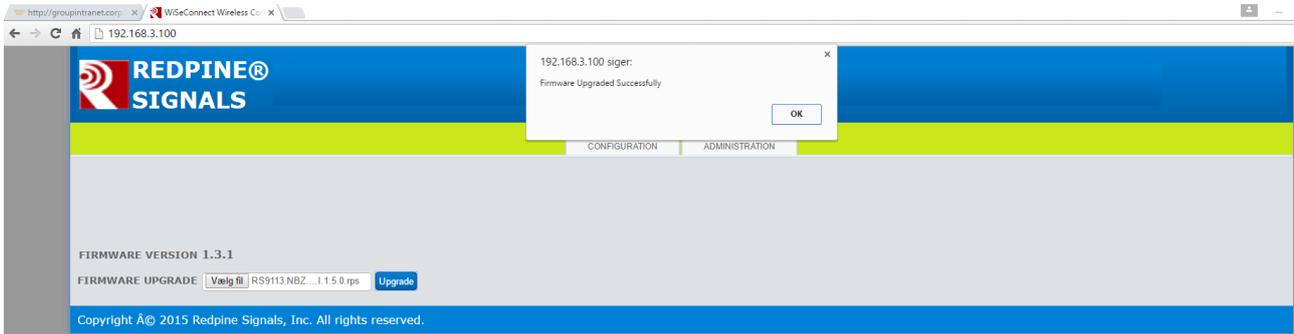
11. When you are prompted "Firmware Upgraded Successfully" and the green flashing stop you have upgraded the firmware. The green light will flash for something like 3 minutes and when it stops you need to restart the unit to make it operational again.
