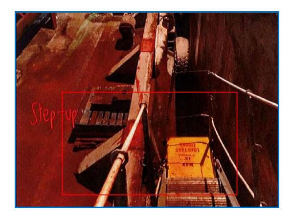
Crewmember overlooked the misalignment of the step-up arrangement as they failed to notice that own vessel had moved ahead and "wooden palette – steps arrangement" need to be readjusted for midship gangway to be readily accessible.
