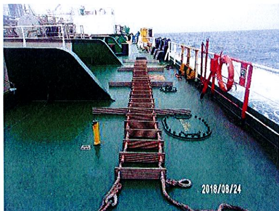
Pilot Ladder(S) Upper
