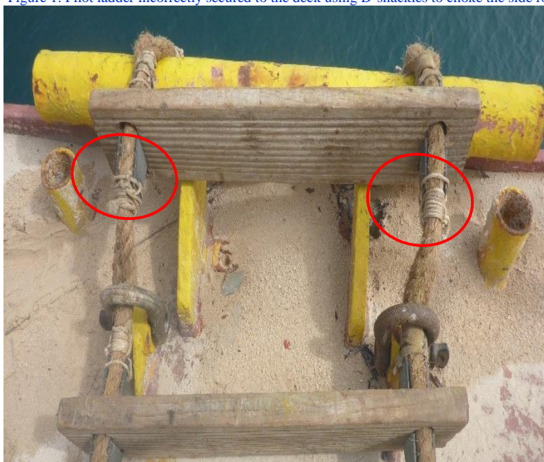
Figure 2. Pilot ladder incorrectly secured to the deck using D-shackles to choke the side ropes
