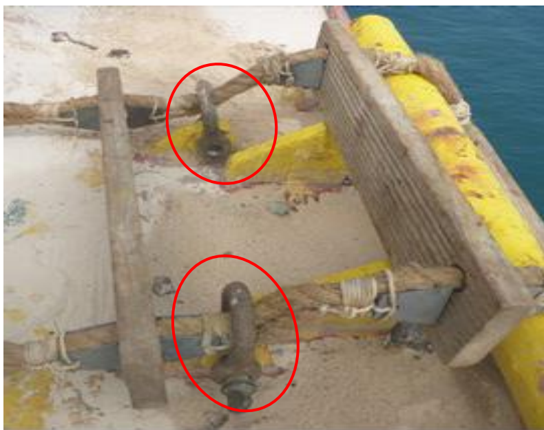
Figure 1. Pilot ladder incorrectly secured to the deck using D-shackles to choke the side ropes
