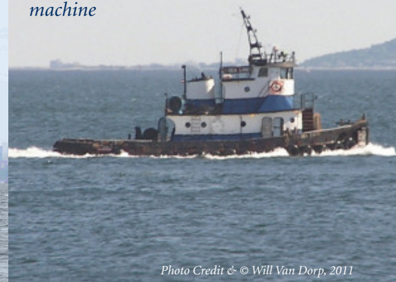
Sea Lion, reportedly a 1,400 horsepower, 38-foot coastwise tugboat with model bow, anchor-handling tug with towing machine
